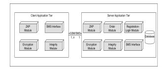
Fig. 3 General structure of the system (2-tier architecture model)
